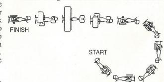
Roll right to upright flight and center the stick to stop the roll.
